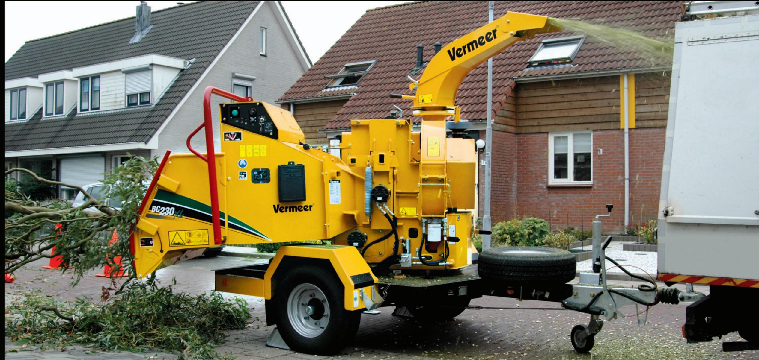
**4: The SmartFeed system.** Increases operator productivity and reduces strain on vital engine parts. A patented feed-sensing control system monitors engine rpm and automatically pauses the rollers when feeding larger material. Additionally, it senses feed-roller jams and responds by automatically reversing infeed and reintroducing the material; this reduces the need for manually manipulating the control bar or the material.
