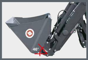
Nothing falls out: Thanks to the excellent tilt angle, there are no trickle losses when loading.
