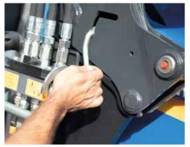
The locking lever is pressed downwards and the front loader securely held in position on the attachment component. Then the front loader is raised higher.
