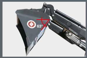
Then the bucket is completely empty – the dump angles for the implement provide efficient results.
