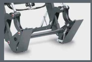
The Skid Steer quick release frame provides a clear view of the implement – ideal when working with the bale spike or pallet fork.
