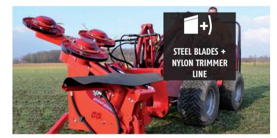
The tractor approaches and the trimmer-head spider with a working width of 0.95m mows down grass under the fence. Due to the central location of the trimmer-head spider, on which three trimmer heads are mounted, it can pivot around its middle axis when working around obstacles (such as posts). It frees obstacles of grass and weeds independently, so there is need to stop the vehicle.
