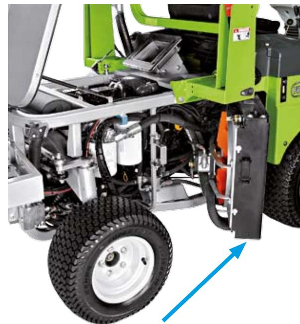
The radiator opens outward to facilitate inspection and cleaning and it is equipped with an automatic system which reverses the rotation of the fan, in order to keep clean the whole surface of the radiator grid, and to guarantee constant control of the temperature. If needed, this operation can also be carried out manually by the operator.
