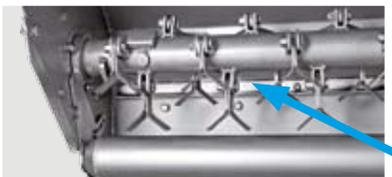
The flail mower comes equipped with a mulching bar, which greatly increases the grass grinding.
