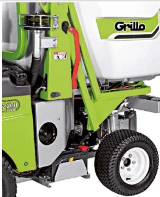
Access to the pre-filter, the engine air filter, the diesel filter and decanter, and the hydraulic oil filter is easy. Even the battery is easily accessed, as well as the belt tensioner and the electromagnetic PTO clutch.
