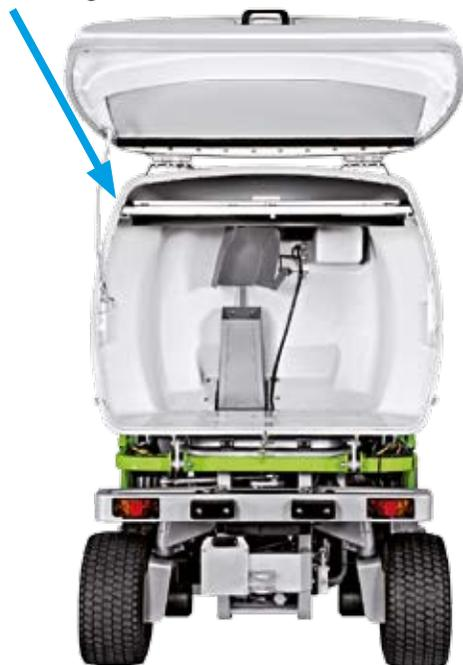
Easy rear access to the hydraulic components such as the variable pump and the service pump.
