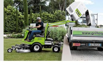
The driver's position of the FD 450 is large, ergonomic and comfortable: the seat is adjustable and dampened in order to adapt to the operator's weight.
