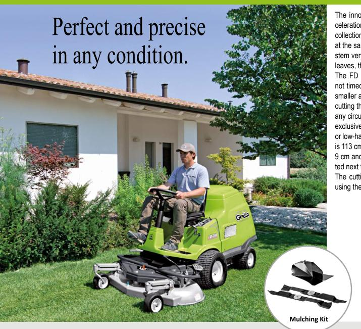
The innovative cutting system "Grillo Overblow" allows an increased acceleration of the grass/air flow into the duct increasing considerably the collection capability, even under conditions of extreme high humidity whilst at the same time keeping the noise level of the whole cutting/collecting system very low. During the autumn season, when the grass is covered with leaves, the FD 280 succeeds in collecting them without blocking.
