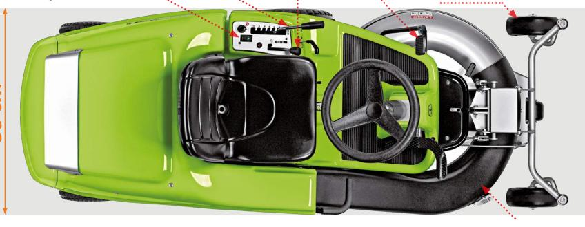
The special blade profile of the FD 220R allows extraordinary cutting and collection even when the grass is humid. This cutting system chops the grass into fine pieces which is then fed directly into the grass catcher through a chute and compacted to reduce its volume. Grass catcher capacity is 200 L.
