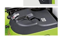
The disc parking brake is of the "active" type: once engaged, it allows you to dismount the machine with the engine running and the cutter disengaged (maximum safety).
