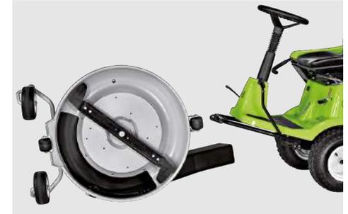
Totally removing the cutting deck is also easy! With a few simple operations it is possible to put it on one side and make it accessible for any service operation such as the replacement of the blade tips or extra cleaning.
