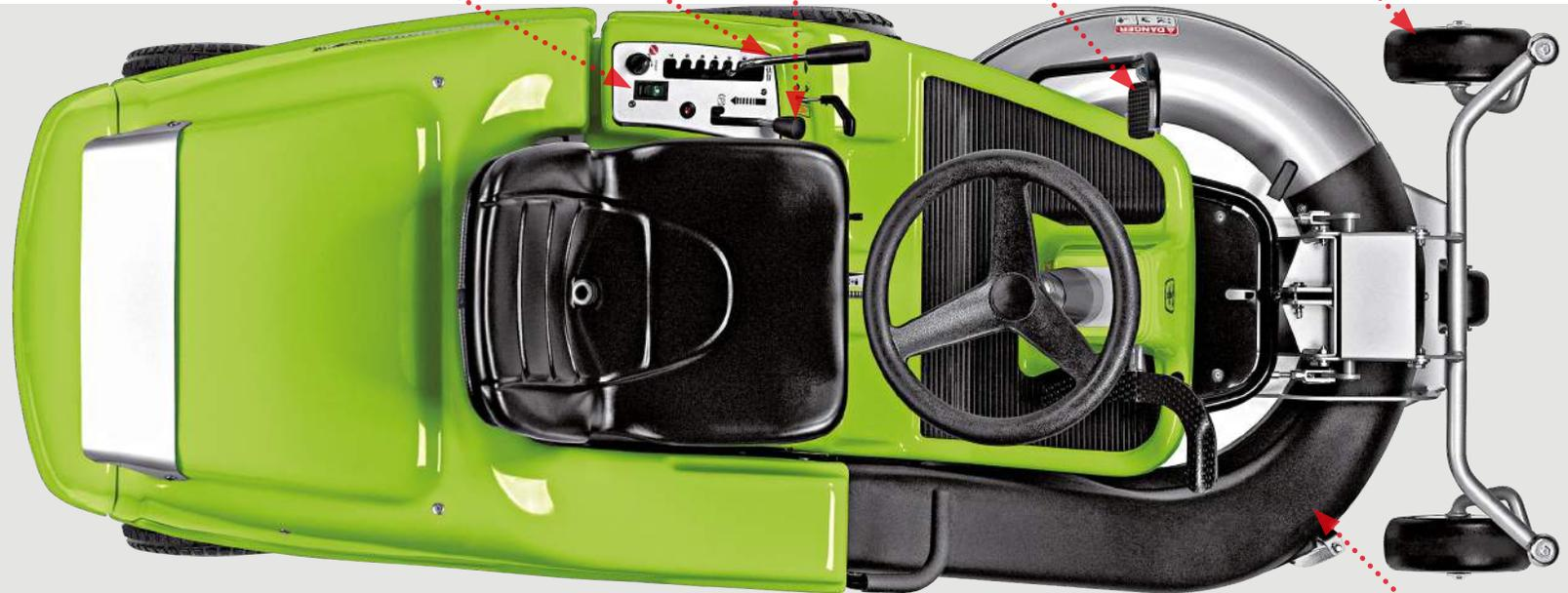
The parking disc brake is controlled by a lever. It allows you to get off the machine with the engine still running and the cutter disengaged (maximum safety).
