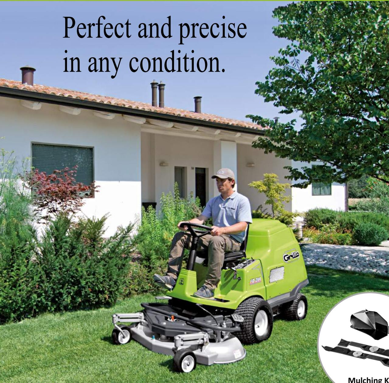
The innovative cutting system “Grillo Overblow” allows an increased acceleration of the grass/air flow into the duct increasing considerably the collection capability, even under conditions of extreme high humidity whilst at the same time keeping the noise level of the whole cutting/collecting system very low. During the autumn season, when the grass is covered with leaves, the FD 280 succeeds in collecting them without blocking.
