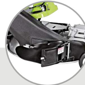
The cutting deck can be converted into a mulch deck or side discharge deck by using the optional kits.
