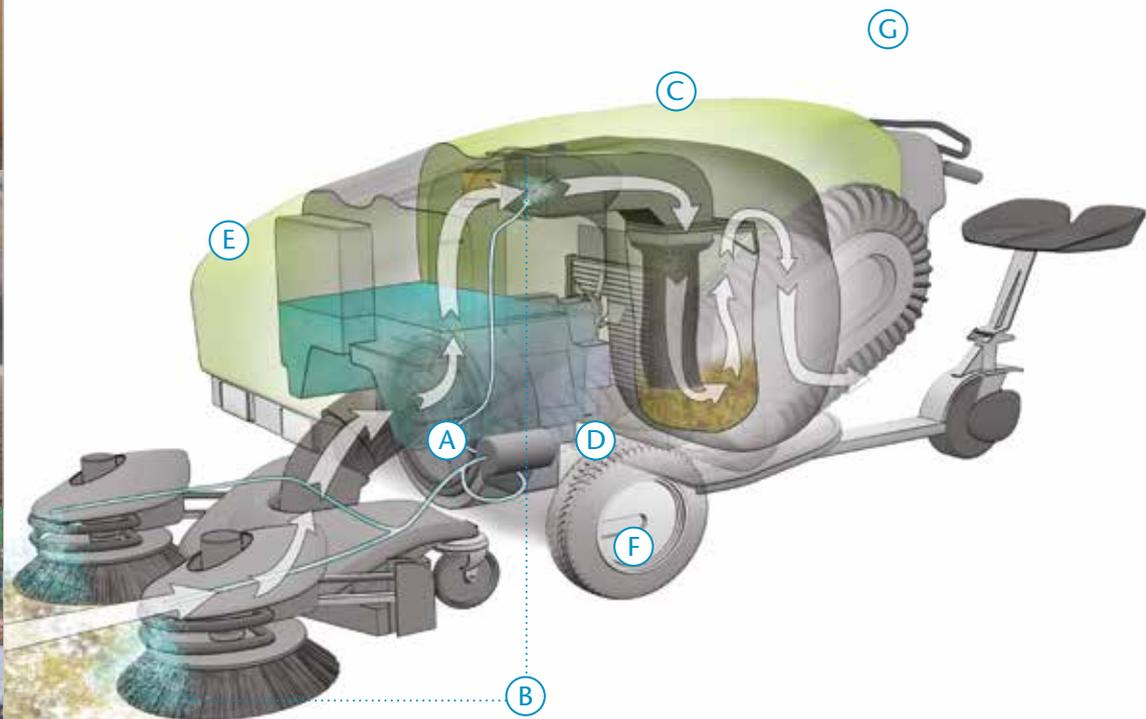
**A** Productivity Boosting Compaction Fan. The 400 Series' pulverising impeller devours debris, reducing leaves and litter to one-third of its original size and broken glass to particles the size of rock salt.
