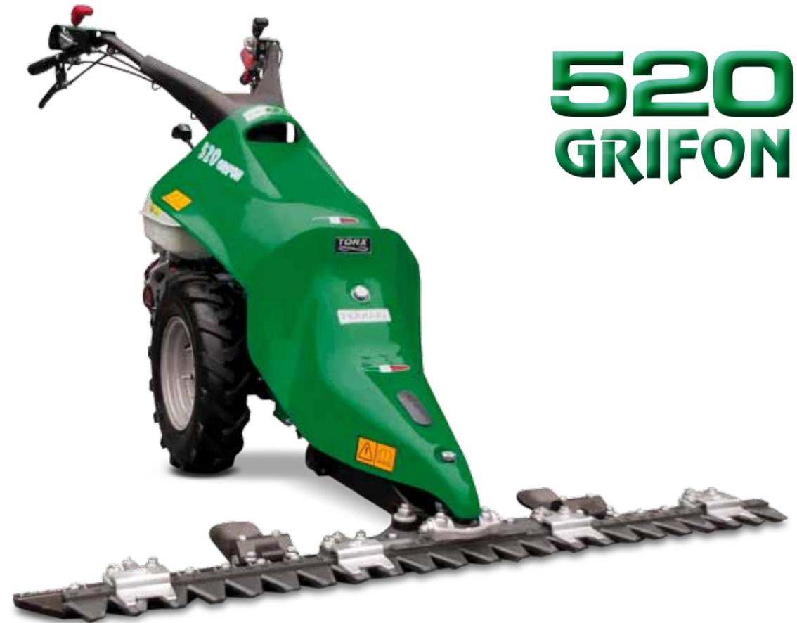
The FERRARI 520 Grifon mowers are equipped with a gasoline engine 8.4 HP Honda GX270 and a 7.5 HP Kohler KD350 diesel engine. The gearbox has four forward speeds, three reverse speeds and a quick reverser. The bars available, from 100 to 180 cm wide, are in the "Laser", "Laser Elasto", with middle cut fingers and Duplex versions. The transmissions, which support and drive the cutter bars, are available in a dry type requiring the usual maintenance and maintenance-free "Torx" models in oil bath.
