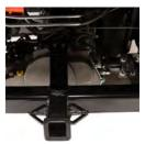
Robust axle mounted hitch with 272 kg (600 lbs) tongue weight and 907 kg (2,200 lbs.) towing capacity (1587 kg (3,500 lbs) with trailer brakes)
