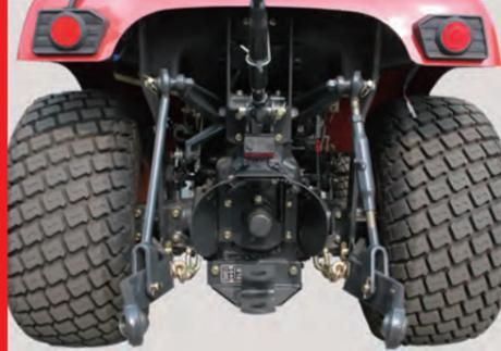
Combined with the rear PTO and SAE category-1 three-point hitch, a variety of implements and attachments can be fitted according to the type of works.
