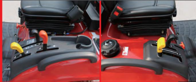
Various levers (HST Hi-Lo range shift, PTO select/clutch, etc.) are arranged either side of the operator seat in an optimal layout to ensure comfortable operation.
