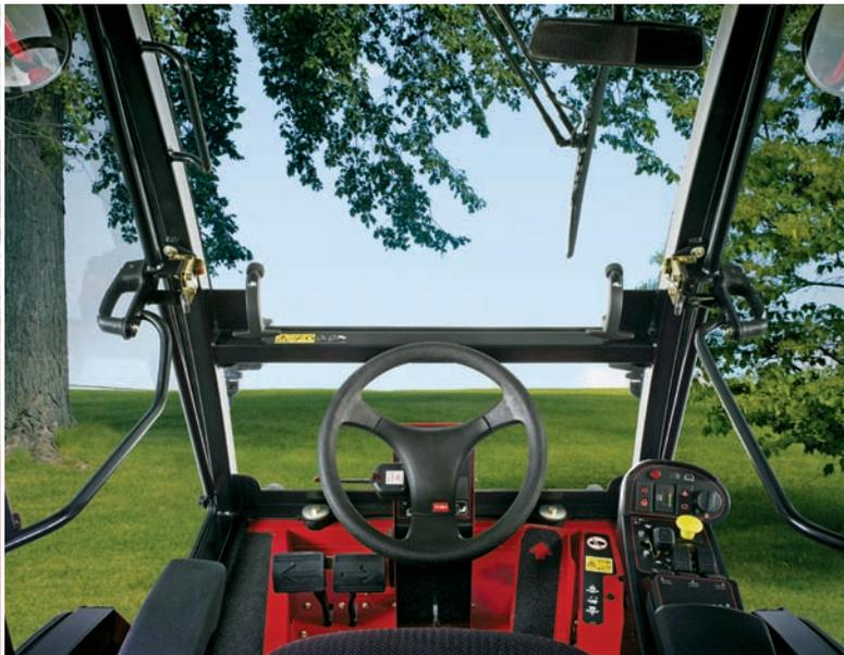
The Groundsmaster 4010-D and 4110-D feature a climate-controlled safety cab, with rollover protection and a pressurized air filtration system that keeps dust and debris away from the operator.
