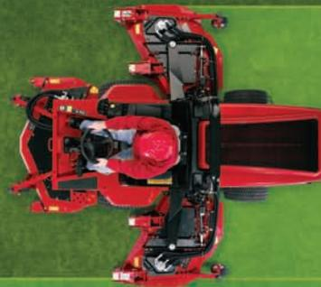
We get what the competition misses. The Groundsmaster 4000-D and 4100-D are engineered to mow a 0" uncut circle without the aid of wheel brakes, so you can easily mow back and forth patterns without missing a blade of grass. Our most nimble large area mowers, the Groundsmaster 4000-D and 4100-D deliver the kind of precision turning that lets you trim around trees and other small objects with one or more decks engaged.
