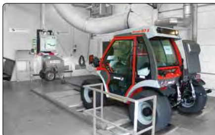
Before delivery, all vehicles undergo intensive functional testing such as here on the chassis dynamometer (pictured).
