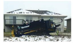
WORTH ITS WEIGHT. Weighing in at 16,500 lb (7484.3 kg), the D23x30pr S3 is the lightest rock drill in its class. The lightweight design helps keep your jobsite intact by decreasing potential disturbance to sidewalks, neighborhoods and landscapes.
