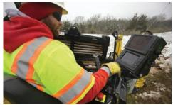
**ROCK QUIETLY.** Following the reliable S3 sound badge, the D23x30pr S3 has an operator ear noise level of 83 dB(A) to help with operator comfort, crew communication and create a guiet working environment to reduce disturbance to neighborhoods and other populated urban areas.
