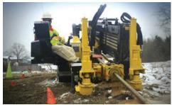
COMPACT CONTROL. A width of 55.5" (141 cm) makes the D23x30pr S3 drill 24.5" (62.2 cm) narrower than its closest competitor, offering efficient maneuverability of the machine into compact urban areas or busy neighborhoods, and convenient transportation on a trailer with other equipment.
