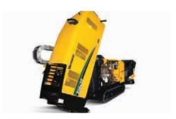
SERVICEABILITY. The drill's flip-up metal hood offers ease of access when performing routine service and maintenance.
