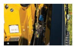
CARRIAGE/VISE SPEED. With a maximum of 130 fpm (39.6 m/min), the carriage speed enables the drill rods to efficiently move up and down the rack.
