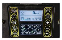
KNOWLEDGE ON DISPLAY. An integrated display allows the operator to optimize machine performance by adjusting operating attachment and ground drive parameters while providing machine diagnostic information including: engine rpm, fuel level, battery voltage, engine coolant temperature and engine hours.
