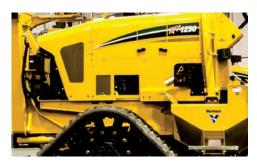
INCREASED POWER. When the RTX1250 engine drops from 2500 rpm to 3000 rpm under load, the horsepower increases from 120 hp (89 kW) to 125 hp (93 kW) allowing the RTX1250 to run at maximum horsepower in work mode.
