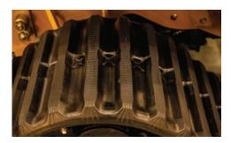
QUAD TRACK SYSTEM. The guad track system offers improved flotation, reduced surface damage and increased tractive effort. Four-wheel steer and crab steering are functional with both quad track and tire options.
