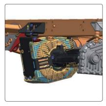
A **wear-free eddy current brake** ensures maximum protection of the service brake and excellent driving comfort even at high load.
