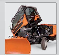
For maintenance in the engine compartment, the **tilting cab** can be hydraulically tilted to the side without tools. Attachments can remain mounted.
