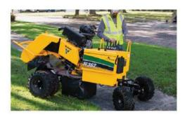
2-SPEED GROUND DRIVE. The operator may choose to operate in a high-range ground speed setting of 67 - 133 fpm (20.4 - 40.5 m/min) to quickly move the machine or choose a slower speed when near the stump by utilizing a low-range setting of 0 - 66 fpm (0 - 20.1 m/min).
