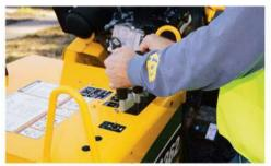
**OPERATOR PRESENCE SYSTEM. Control** handles for boom swing, boom raise/lower and machine propel are equipped with an operator presence feature. This user-friendly operator presence system is intended to enhance operator safety.
