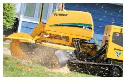
PRODUCTIVE CHIPPING. With a 67 hp (50 kW) Cat C2.2L turbocharged Tier 4 Final/Stage IIIB diesel engine, this machine is ready for tough cutting jobs.
