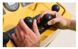
**OPERATOR PRESENCE SYSTEM.** This operator system is intended to help protect the operator. If the operator's hand(s) leave the cutter wheel controls for more than one second, the cutter wheel will disengage, come to a stop and the cutter wheel indicator light will go out.
