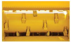
**DUPLEX DRUM.** To reduce daily maintenance time, the patented duplex drum, designed with reversible tips and hammers, is available.
