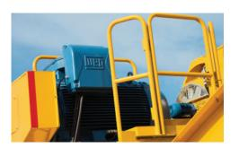
**ELECTRIC MOTORS.** Equipped with a 500 hp (373 kW) WEG totally enclosed, fan-cooled electric motor to power the mill. A separate 50 hp (37 kW) electric motor powers the pump for the hydraulic circuits, while a 2 hp (1 kW) electric motor powers the fan to cool the hydraulic system.
