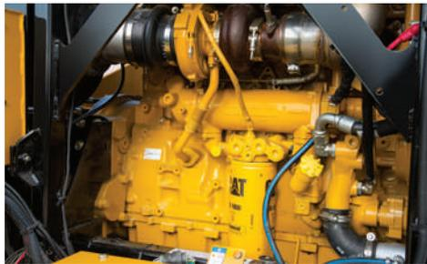
**ENGINE POWER.** A CAT C13 Tier 4 Final engine provides 440 hp (328 kW) of power to meet your jobsite demands. A Tier 3 engine option is available for less-regulated countries.
