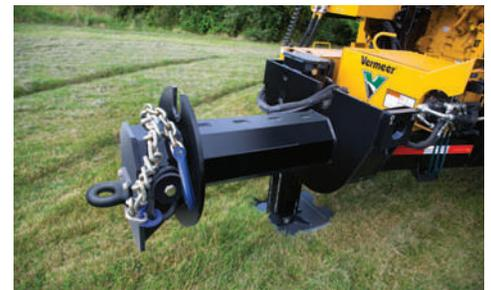
**JOBSITE MOBILITY.** The WC2300XL has a compact design and built-in skidder grab on the tongue, allowing it to be moved around on the jobsite by a skidder or excavator.
