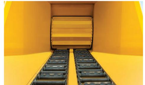
**INCREASE PRODUCTIVITY.** With technology such as SmartCrush to automatically increase down pressure when difficult material enters the cutting drum, and the variable-speed dual-infeed conveyor chains, operators can concentrate on loading the machine, not pushing the material through.
