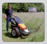
The twin blade mower with lateral drive is especially suited for mowing along embankments and guard rails.
