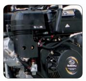
A powerful four stroke Robin EH 41 engine with 9.9 kW (13.5 hp) provides the necessary power for every situation
