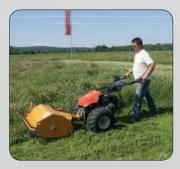
The cutting height of the **FMF 80 flail mower** with rear roller is adjustable from 45 to 110 mm.
