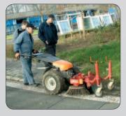
Weeder WE 100 with counter rotating disk or cup brushes and support wheels for cleaning up and tidying pavements and kerbs.
