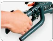
**Finger guards** are highly desirable when operating the machine alongside shrubs or other obstructions.
