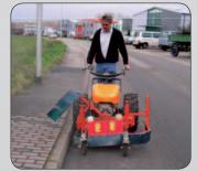
Weeder WE 90 with counter rotating disk or cup brushes and support wheels for cleaning pavements and kerbs.
