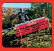
Belt rake BR 3/10 / BR 3/11 with support wheel steering, working width 160 and 180 cm
