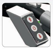
**Electro hydraulic travelling drive adjustment.** You can conveniently adjust your operating speed at the push of a button by using the directional touch pad.
