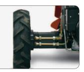
The **wide gauge assembly** is 280 mm wider and is excellent for slopes and cross country applications (only for M14).
