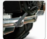
**Standard M14 axle adjustment** allows you set the best possible weight distribution for the various implements and working conditions.
