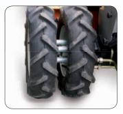
can be equipped with the high grip 5.0-10 AS
