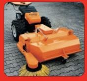
**Combi sweeping machine 2350** heavyweight version, 110 and 130 cm, 2 speeds, support rollers, swivelling. Optional: dirt holder, side broom
