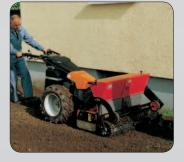
The SM 75/90 and 100M add on seeding machines for the rotary harrow provides even sowing. The sowing shaft is driven via the grid roller.
