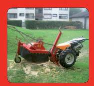
Tree stump grinder SF 50 with hardened cutter wheel, disk diameter: 50 cm
