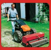
Path maintenance machine WP 75 / 90 / 100 with adjustable grid roller, working width 75, 90 and 100 cm
