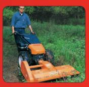
Safety mulcher SM 90 / 105 / 125 with rear roller and spiral shaft, working width 90, 105 and 125 cm
