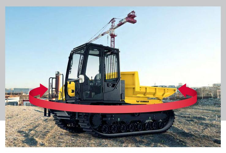
The total mass of the C50R-5A is evenly distributed on the ground via 32 rollers. Fully loaded, the machine has a ground pressure as little as 32,4 kPA. This improves the all-terrain capabilities drastically and the C50R-5A can work in the worst ground conditions.
