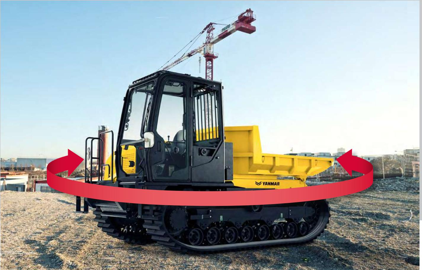
The total mass of the C50R-5A is evenly distributed on the ground via 32 rollers. Fully loaded, the machine has a ground pressure as little as 32,4 kPa. This improves the all-terrain capabilities drastically and the C50R-5A can work in the worst ground conditions.
