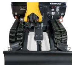
Retracted undercarriage : 980 mm
