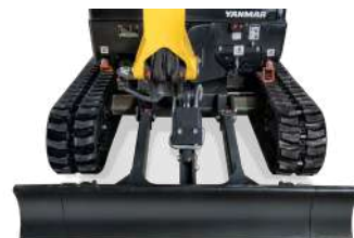
Extended undercarriage: 1380 mm
