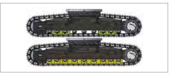
**Track guards:** to provide better protection, track alignment, and performance of machine while travelling. 3 guards per track as standard or DX490LC-7 & DX530LC-7 (full-length track guard optional) and, for DX420LC-7, 2 guards per track as standard (double and full-length track guards available as options). These various track guard options provide you with optimal solutions for your extreme applications.
