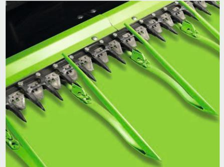
⬆ The offset configuration of the knife sections reduce wear and ensures excellent cutting results in all conditions.
