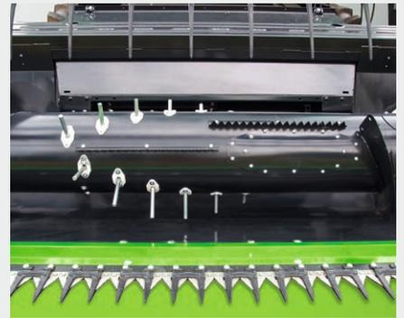
⬆ The feeder auger with full length retractable fingers ensure continuous feed and crop flow.
