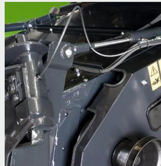
↑ Adjustable cutting angle for following the contours of uneven terrain perfectly.
