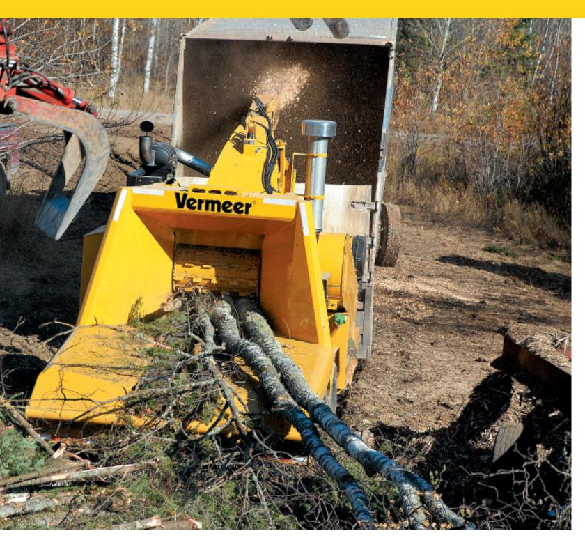
**Dual-knife options.** The drum and cutter design provides two different depths of cut, 3/8" (.8 cm) and 5/8" (1.6 cm). This allows one machine to provide different end products to meet customers' needs.
