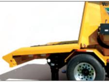
**Sloped infeed table.** A six-degree sloped infeed table lowers the "break-over" point where long material first contacts the machine. This provides smooth flow of long material from the ground up onto the infeed table and reduces the likelihood of limbs or tree canopy from snagging on the end of the machine.
