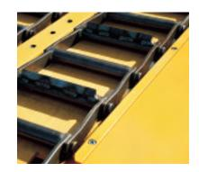
**Replaceable wear components.** High-wear material flow areas of the machine, such as the drum, discharge chute, cutter housing and infeed conveyor floor are designed with replaceable bolt-in wear parts to extend machine life.
