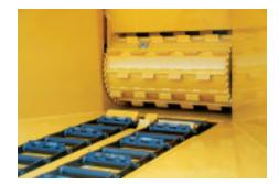
**Infeed system.** The WC2300 features an infeed system that includes variablespeed dual infeed conveyor chains, conveyor head pulley with integral grip bars, sloped infeed table and aggressive infeed roller with crush capability. These provide efficient feeding of difficult material types, reducing the number of times an operator has to handle the material.
