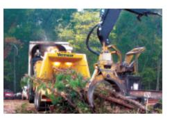
**Ecoldle™.** When the Ecoldle function is selected, the engine speed automatically lowers to 1400 rpm after 30 seconds of inactivity to help reduce fuel consumption when not chipping material.
