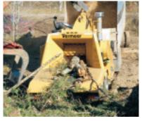
**SmartCrush.** The machine monitors the position of the infeed roller. Down pressure is off until the feed roller has climbed up onto the material, then increases to crush difficult material with forks or large limbs to the cutter drum. With material securely gripped by the infeed system, the operator can release the grapple and concentrate on the next load of material.
