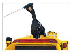
An optional patent-pending winch eliminates the need to drag large material to the chipper. The 150' (45.7 m) winch line can handle material up to 4000 lb (1814.9 kg), making it easy to lift logs directly onto the feed table. In addition the winch can also be hydraulically raised out of the way to allow operators to feed the unit using a loader.
