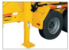
**Optional hydraulic outriggers** support the back of the chipper and prevent the unit from bouncing while chipping or loading large-diameter material onto the feed table.
