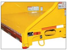
Bottom feed stop bar is strategically located to make it possible for the operator to strike the bar and shut off the feed either intentionally or automatically in an emergency situation. A reset button on each side of the infeed housing allows for easy system reset if the bar is tripped.
