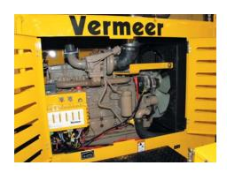
**Three Cummins diesel engine options** to match most jobsite needs.
