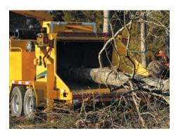
SmartCrush puts the pressure on branches. Once the upper feed roller raises for four seconds, it will automatically increase down pressure on the material being fed. This allows the upper feed roller to easily climb onto large forked material before the increased down pressure is applied for maximum pulling force.
