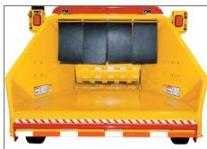
**The infeed table design** is the largest in its class! It funnels material to the drum opening, allowing for smooth material feeding from table to drum. The overall table width is 72" (182.9 cm) with a 39" x 62" (99.1 cm x 157.5 cm) opening by the infeed curtains and a drum opening of 21.5" x 28" (54.6 cm x 71.1 cm).
