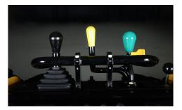
**JOYSTICK CONTROL.** Operators can steer with a single pilot-operated joystick. The single joystick offers the operator a smooth range of motion without balancing engagement of two separate controls.
