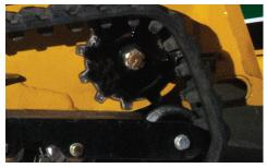
**LOWER YOUR COST OF OPERATION.** The undercarriage features a high track-mounted sprocket. The higher mounting reduces premature wear and tear in rocky soil conditions, while the ADI cast sprocket is heat-treated for longer life.
