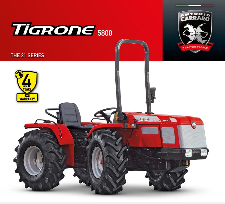
The **Tigrone 5800** is a new equal wheel tractor from the unbeatable Series 21. Designed for work on hillsides and mountains and specialised crops. Four equal wheel drive, optimum weight-power ratio, reduced steering angle all mean stability and constant traction on all types of terrain along with a capacity for quick manoeuvrability and disengagement.
