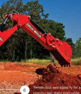
best-in-class static load rating of 39,000 lb (17,690 kg) and best-in-class 35,215 lb (13,944 kg) of breakout for plowing applications.
