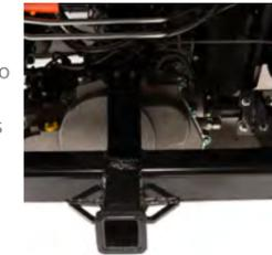
**Robust axle mounted hitch** with 272 kg (600 lbs) tongue weight and 907 kg (2,200 lbs.) towing capacity (1587 kg (3,500 lbs) with trailer brakes)
