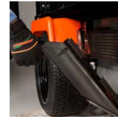
**Tool-less access to the radiator** and optional hydraulic oil cooler for easy cleaning
