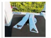
HYDROSTATIC TRANSMISSION with double pedal (forward/ reverse) and two forward speed ranges.
