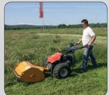
The cutting height of the **FMF 80 flail mower** with rear roller is adjustable from 45 to 110 mm.
