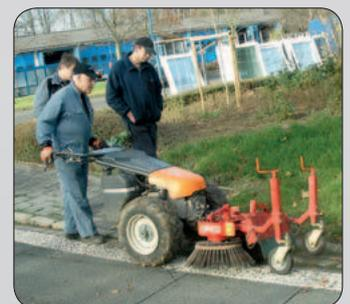
**Weeder WE 100** with counter rotating disk or cup brushes and support wheels for cleaning up and tidying pavements and kerbs.
