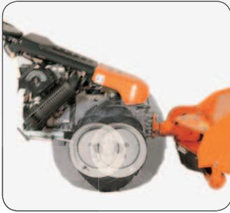
**Standard M14 axle adjustment** allows you set the best possible weight distribution for the various implements and working conditions.
