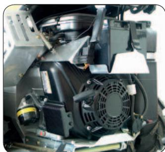
The M14 has a powerful 2-cylinder 4-stroke petrol engine which offers both power and endurance. 15.4 kW (21 hp). With optional electric starter!
