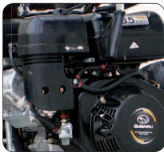
A powerful four stroke Robin EH 41 engine with 9.9 kW (13.5 hp) provides the necessary power for every situation
