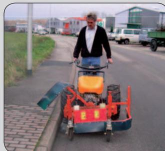
**Weeder WE 90** with counter rotating disk or cup brushes and support wheels for cleaning pavements and kerbs.
