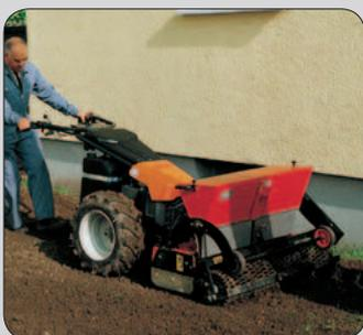
**The SM 75/90 and 100M** add on seeding machines for the rotary harrow provides even sowing. The sowing shaft is driven via the grid roller.
