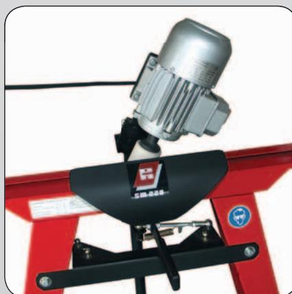
**Double-knife cutter drive with blade protection**
