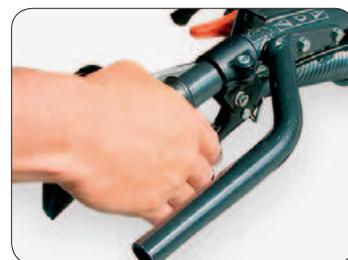
**Finger guards** are highly desirable when operating the machine alongside shrubs or other obstructions.
