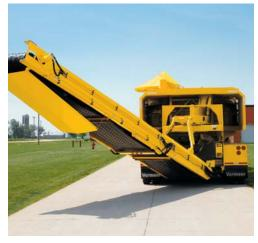
Radial stacking conveyor. The rear uploading conveyor oscillates 60 degrees allowing the operator to change placement of the processed material without moving the machine. The conveyor may be equipped with an optional magnetic head pulley to help remove steel metallic materials, resulting in a more useful end product.
